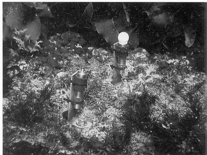
Fig. 3. Measurements of light quantity and water temperature by data loggers.
