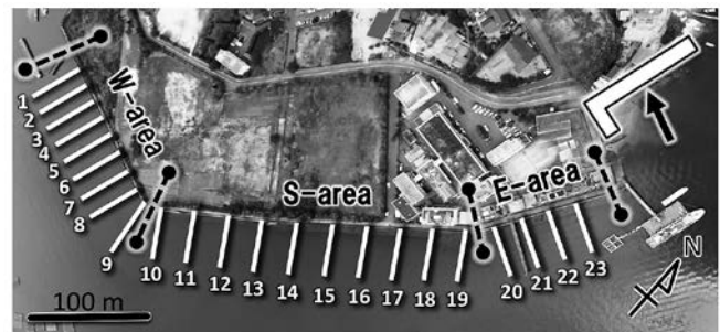
Fig. 2. Arrangement of survey lines with the bottom topography along the stone-built seawall mound at the study site. Arrow shows the new seawall mound after first survey in this study.
